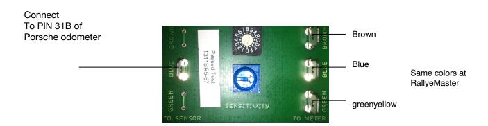
Mount the interface behind the odometer. Please check, that there is no connection to other parts!
